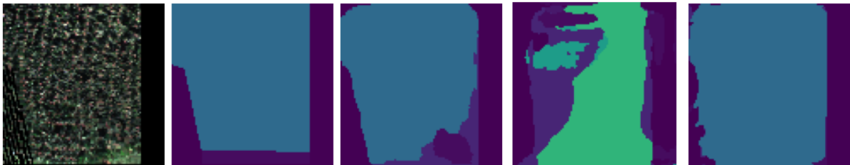
Figure 39: The visualization shows an example of semantic segmentation from our model using an image from UAV-HSI-CropDataset. (a) RGB, (b) ground-truth, (c) Our HRViTUNet fine-tuned on this agricultural HSI dataset, (d) TransUNet fine-tuned on RGB dataset, (e) TransUNet fine-tuned on HSI dataset.
